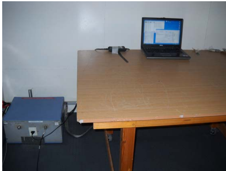
Photograph 7.1.1 Setup for conducted emission measurements
