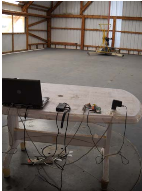
Photograph 7.2.3 Setup for radiated emission measurements at OATS, EUT cabling
