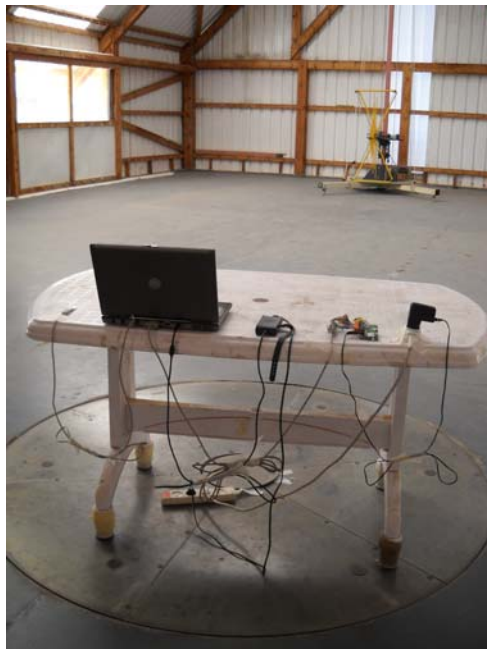
Photograph 7.2.3 Setup for radiated emission measurements at OATS, EUT cabling
