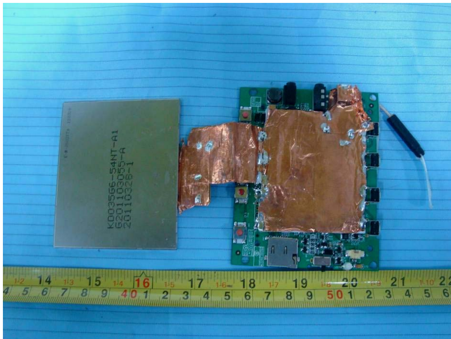
EUT – Main Board with LCD Top View
