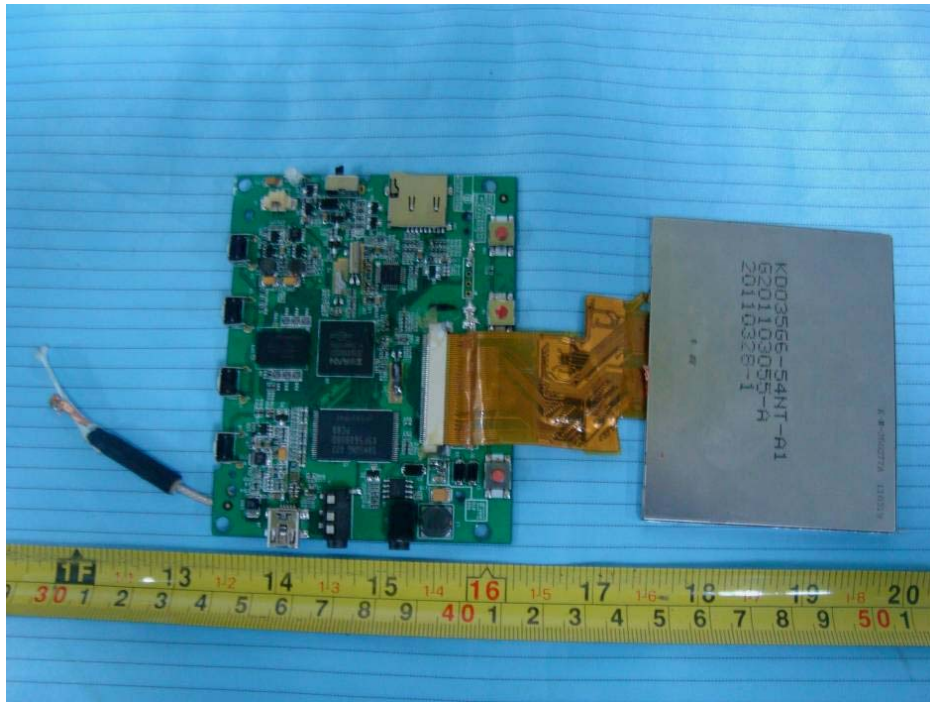
EUT – Main Board with LCD Bottom View
