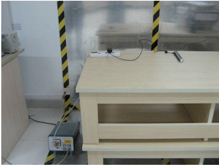
FCC RADIATED EMISSION TEST SETUP
