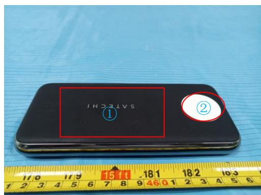
① Wireless charging area for mobile phone which include one coil.
