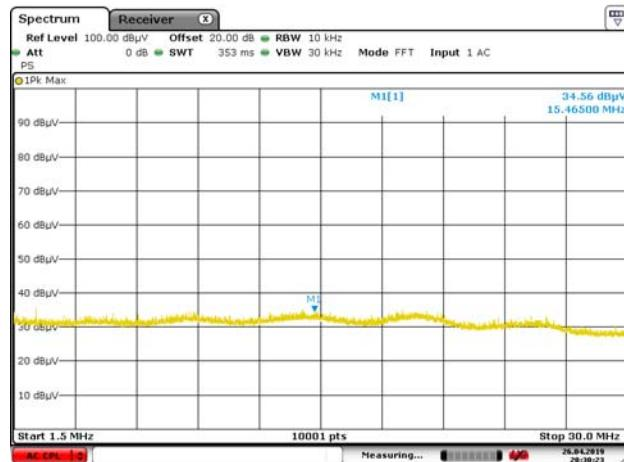
Remark: during the measurements, the correction factor (antenna factor and cable loss) was compensated as Offset 20 dB.
