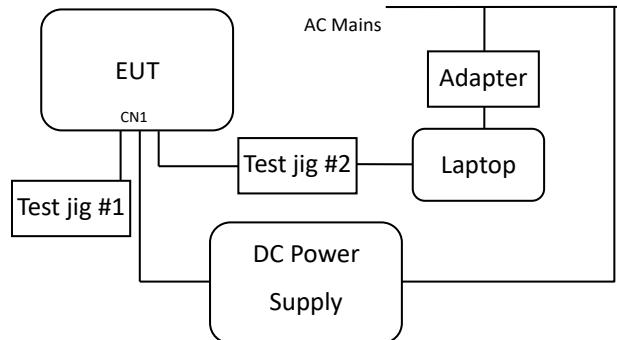
NOTE: The Test jig #1 was connected for the normal operation for the transceiver operating at 2405 MHz.
