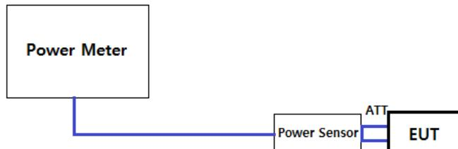
Note 1: The conducted average power was measured using a wideband gated RF power meter and gate parameters was adjusted such that the power is measured only when the EUT is transmitting at its maximum power.
