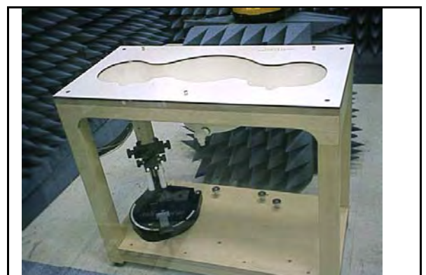
Figure 6. SAM Twin Phantom
