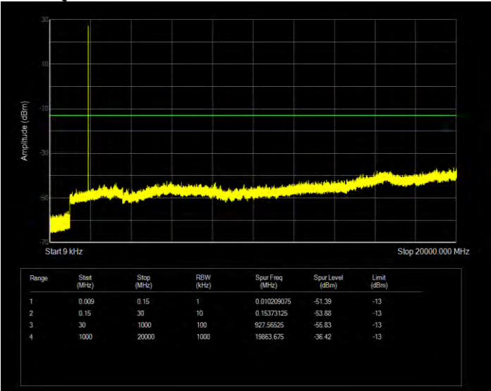
Band2 16QAM BW=1.4MHz Channel=19193 RB Size=1 Position=#0
