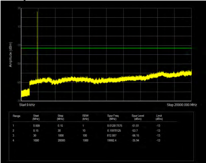
Band2 QPSK BW=3MHz Channel=19185 RB Size=1 Position=#0
