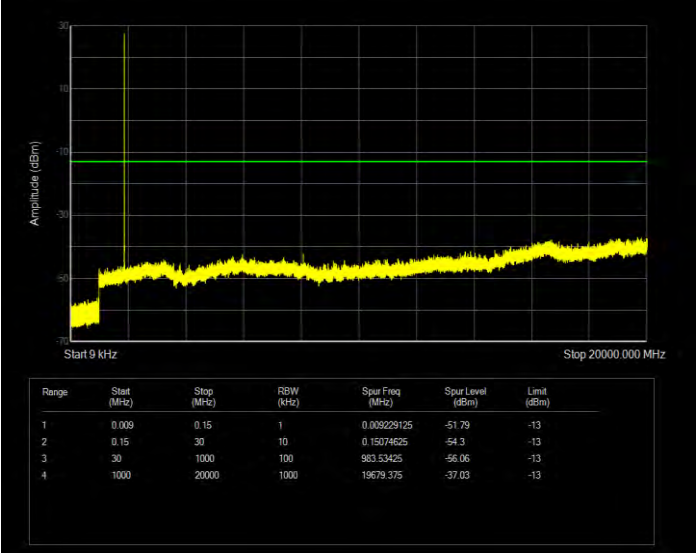
Band2 16QAM BW=1.4MHz Channel=19193 RB Size=1 Position=#0
