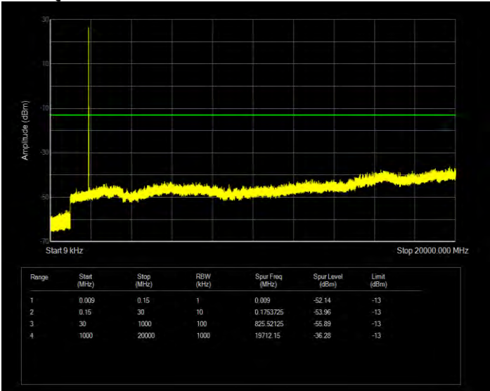
Band2 QPSK BW=5MHz Channel=19175 RB Size=1 Position=#0
