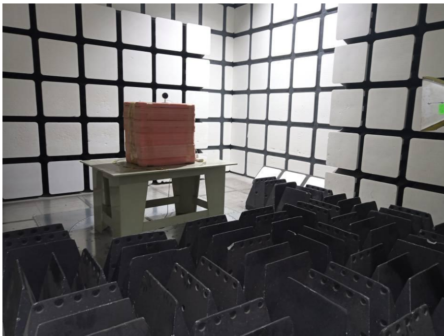
Radiated Emissions View (Above 1 GHz)
