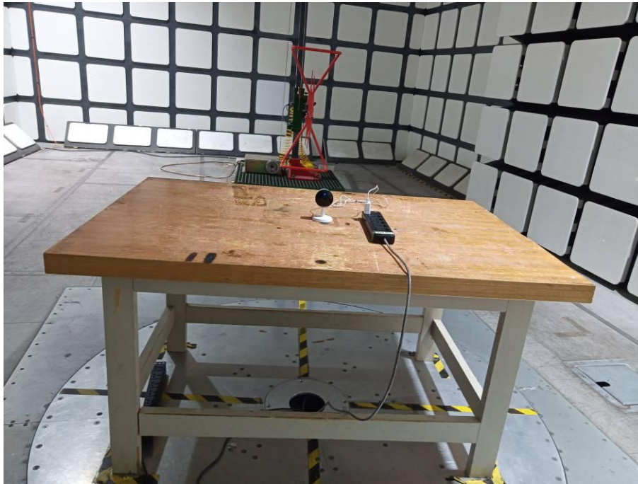
Radiated Emissions View (Below 1 GHz)
