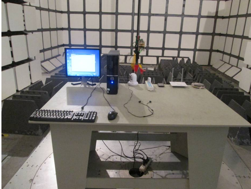
Radiated Emissions – Front View (Above 1 GHz)
