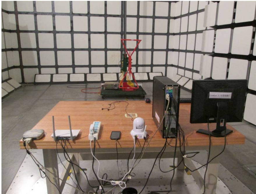
Radiated Emissions – Rear View (Below 1 GHz)
