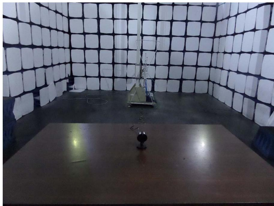
**Radiation Emission Test Setup (Above 1GHz)**
