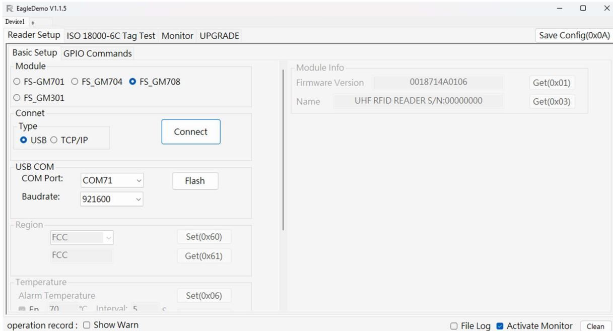
2.1.2. Please select **USB** as **Connection**, Choose the corresponding **Serial Port** and **Baud Rate** (default baud rate is 921600). As illustrated below:
