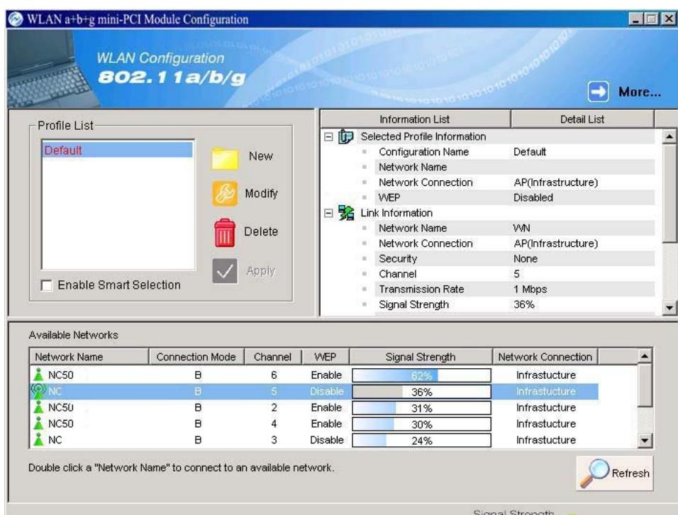
**Note!** To automatically connect to the network with the strongest signal, select **Enable Smart Selection**. **Any** displays in Profile List.
