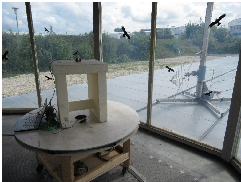
Open area test site, 30 MHz - 1000 MHz
