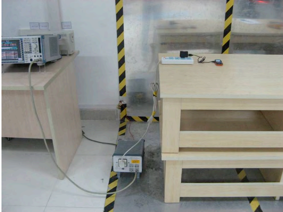
RADIATED EMISSION TEST SETUP
