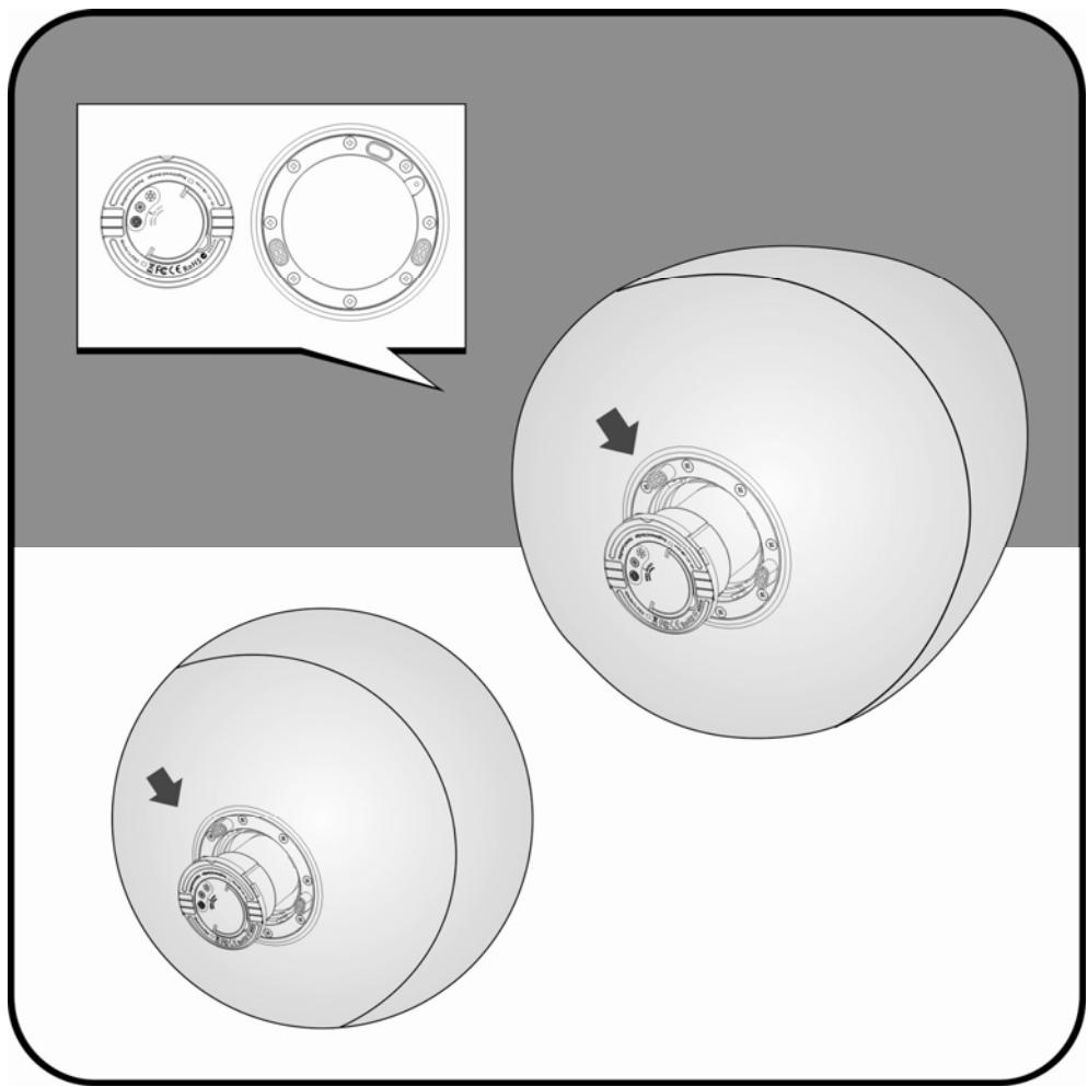
**Once removed the LED module, do not try to open it : This will void the warranty**
