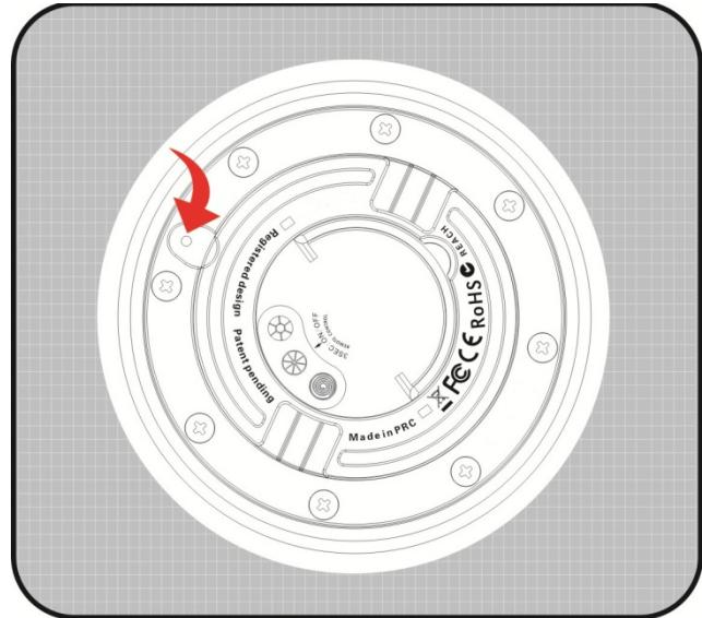
Step 2: slowly twist the LED module from left to right (clockwise to unlock the led module). You can use the small metal hook underneath the led module to help you.
