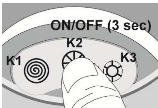
**You can switch ON and OFF the remote controller receiver inside the Led module pressing 3 seconds the button K2 underneath the LED module.**
