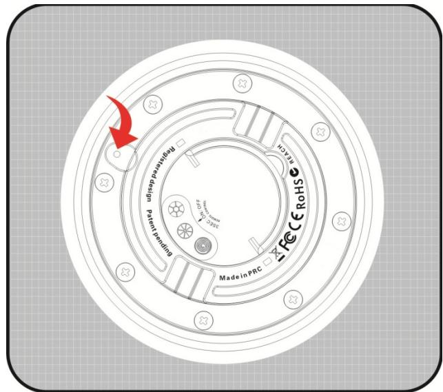
Step 2: slowly twist the LED module from left to right (clockwise to unlock the led module). You can use the small metal hook underneath the led module to help you.
