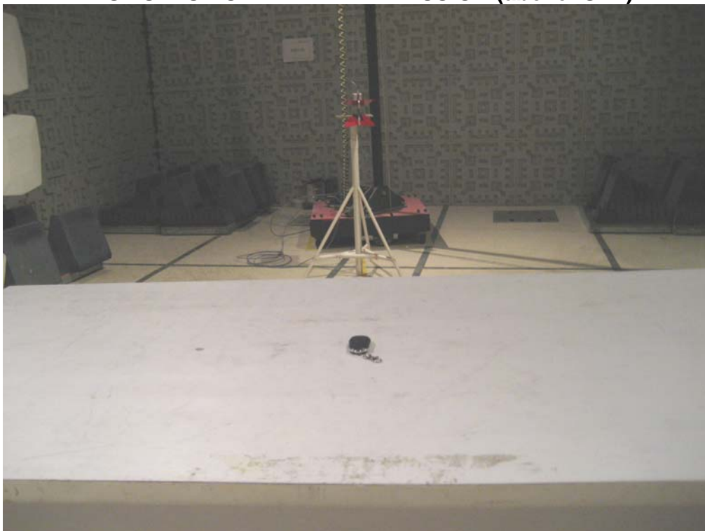
TEST SETUP OF RADIATED EMISSION (above1GHz)
