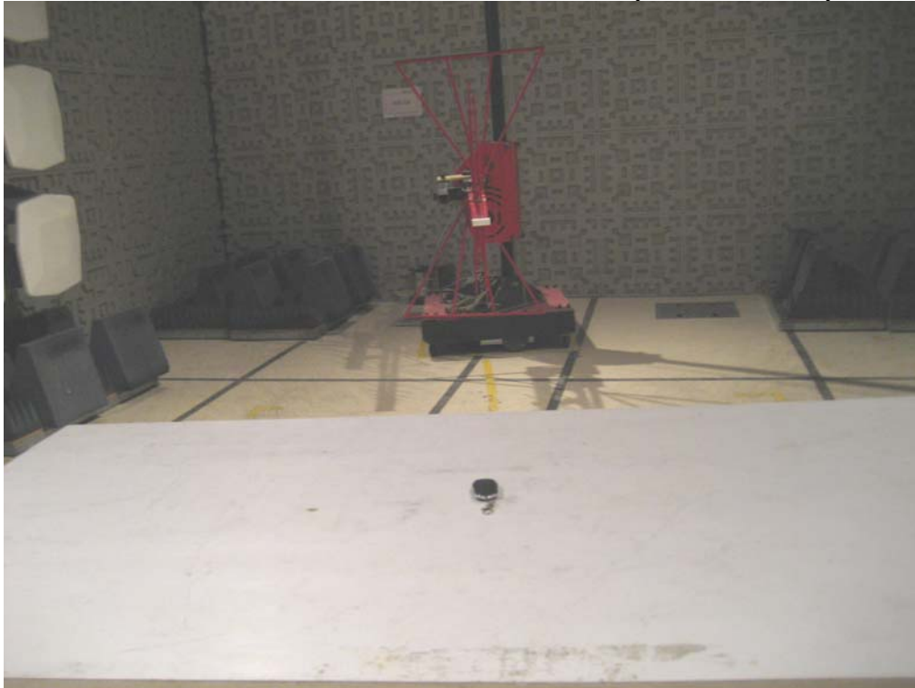
TEST SETUP OF RADIATED EMISSION (30MHz -1GHz)
