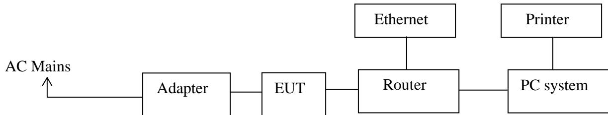
6.1.2. Semi-anechoic Chamber Test Setup Diagram
