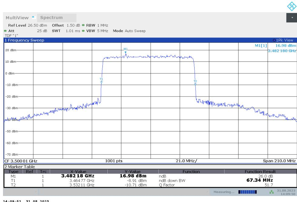
n78L,70MHz Bandwidth,DFT-s-QPSK (-26dBc BW)
