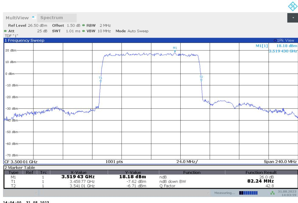
n77L,80MHz Bandwidth,DFT-s-QPSK (-26dBc BW)
