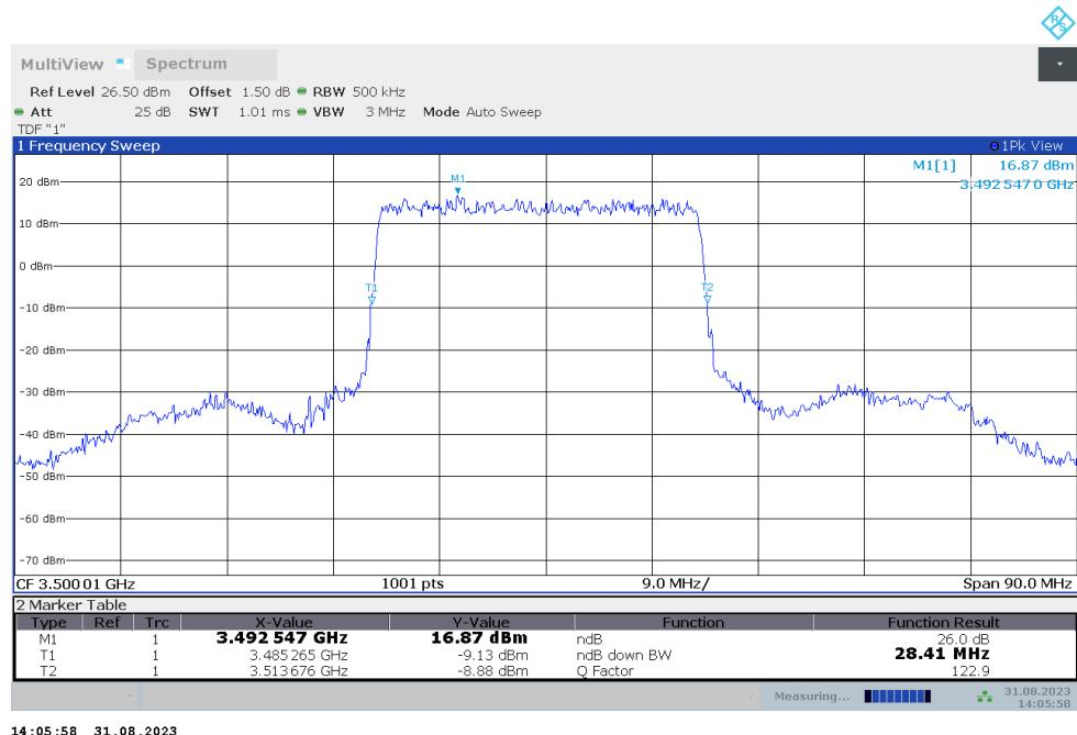
n78L,30MHz Bandwidth,DFT-s-QPSK (-26dBc BW)
