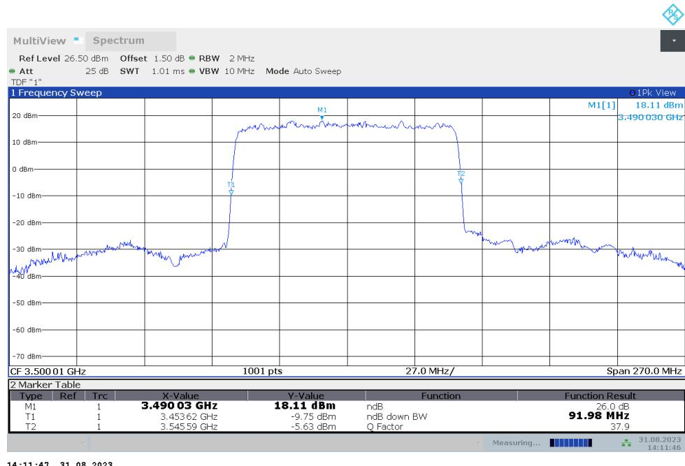
**n78L,90MHz Bandwidth,DFT-s-QPSK (-26dBc BW)**
