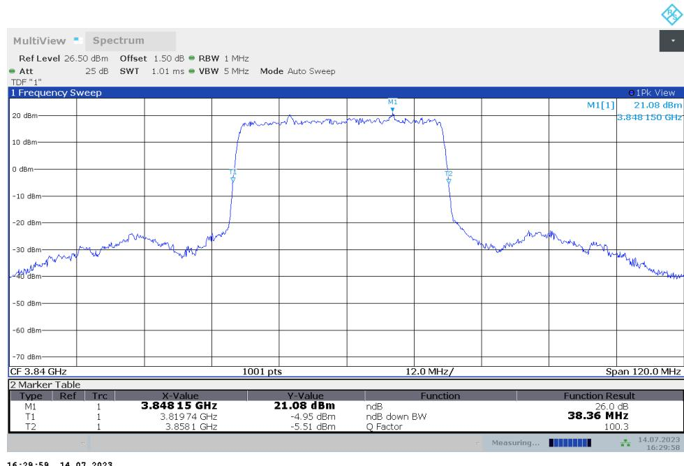
**n77H,40MHz Bandwidth,DFT-s-QPSK (-26dBc BW)**
