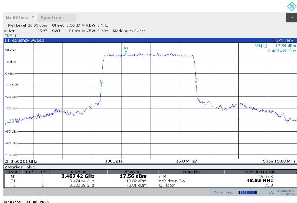
**n78L,50MHz Bandwidth,DFT-s-QPSK (-26dBc BW)**
