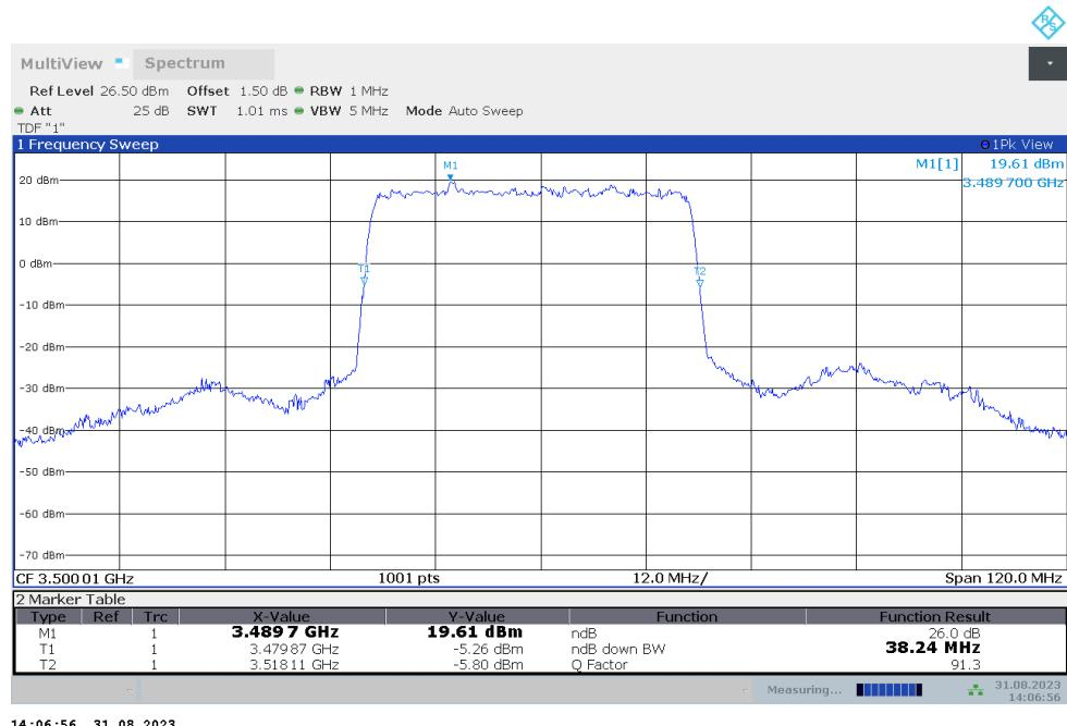
**n78L,40MHz Bandwidth,DFT-s-QPSK (-26dBc BW)**
