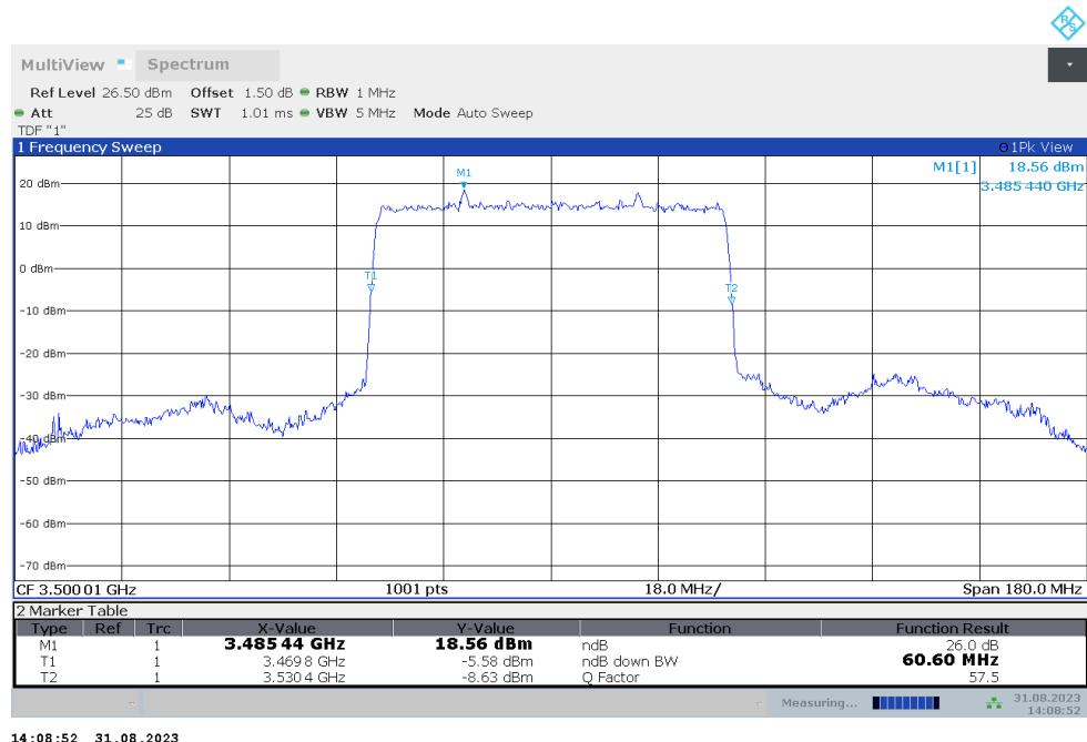
n78L,60MHz Bandwidth,DFT-s-QPSK (-26dBc BW)
