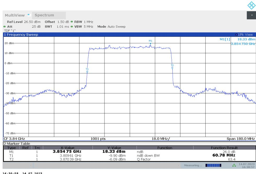
**n77H,60MHz Bandwidth,DFT-s-QPSK (-26dBc BW)**
