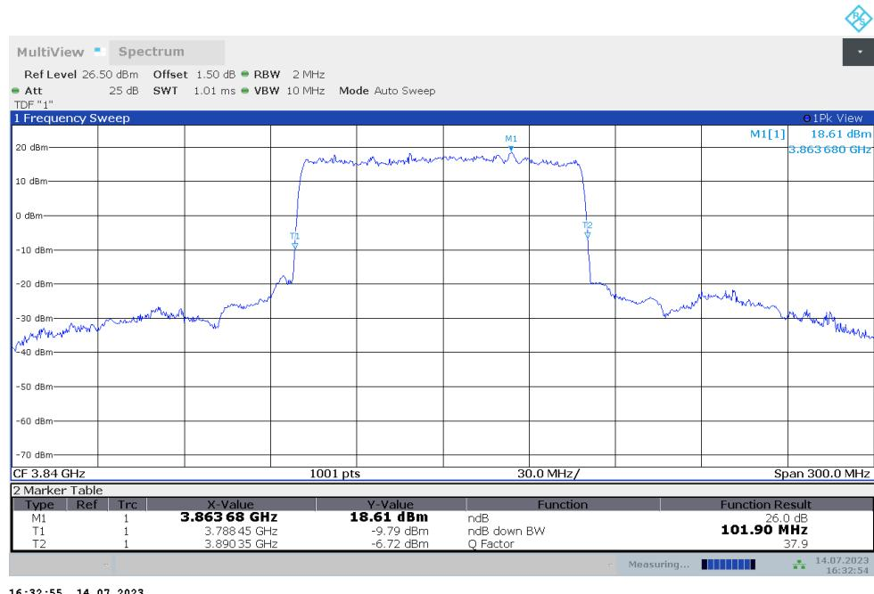
**n77H,100MHz Bandwidth,DFT-s-QPSK (-26dBc BW)**
