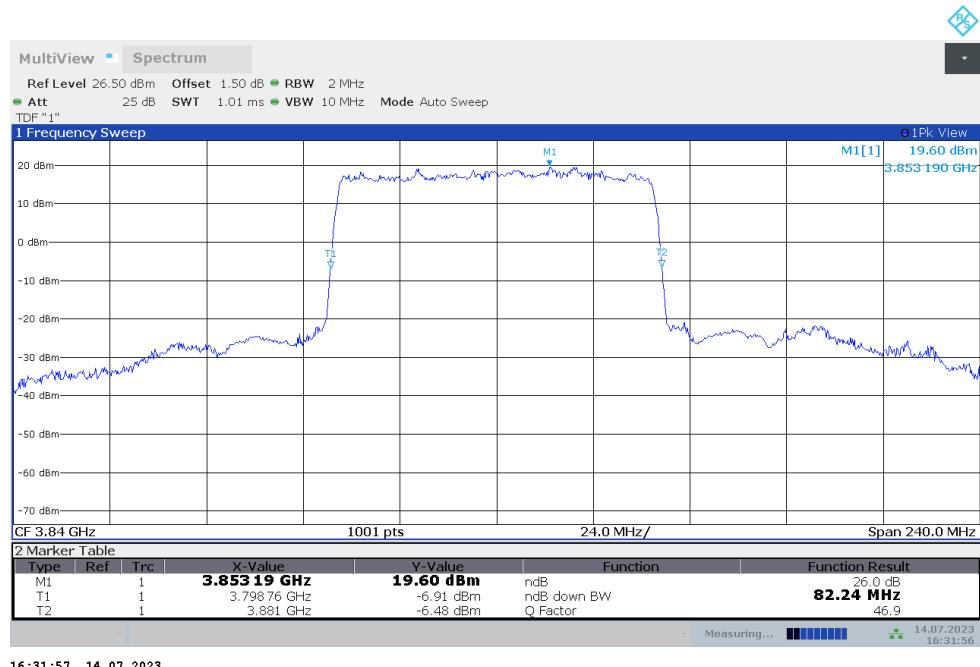
n77H,80MHz Bandwidth,DFT-s-QPSK (-26dBc BW)
