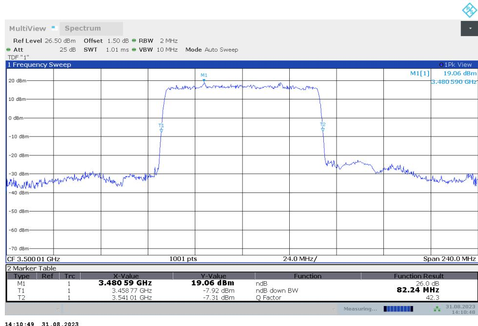
**n78L,80MHz Bandwidth,DFT-s-QPSK (-26dBc BW)**
