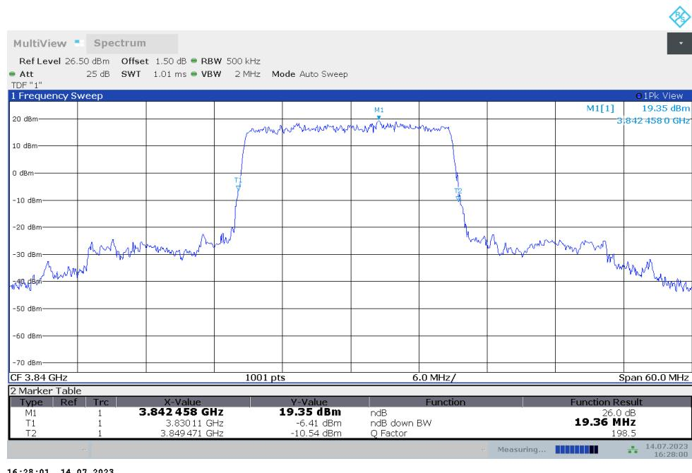
**n77H,20MHz Bandwidth,DFT-s-QPSK (-26dBc BW)**
