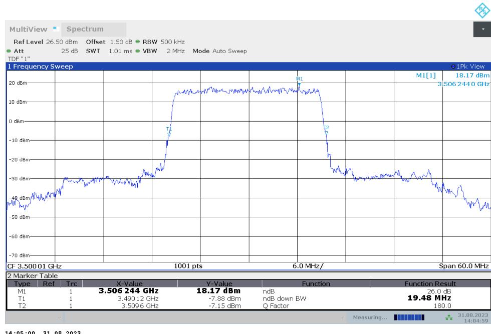
**n78L,20MHz Bandwidth,DFT-s-QPSK (-26dBc BW)**
