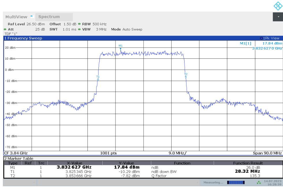
**n77H,30MHz Bandwidth,DFT-s-QPSK (-26dBc BW)**
