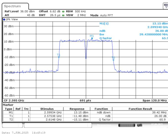
**LTE CA band 38C , 20MHz+20MHz Bandwidth,16QAM (-26dBc BW)**
