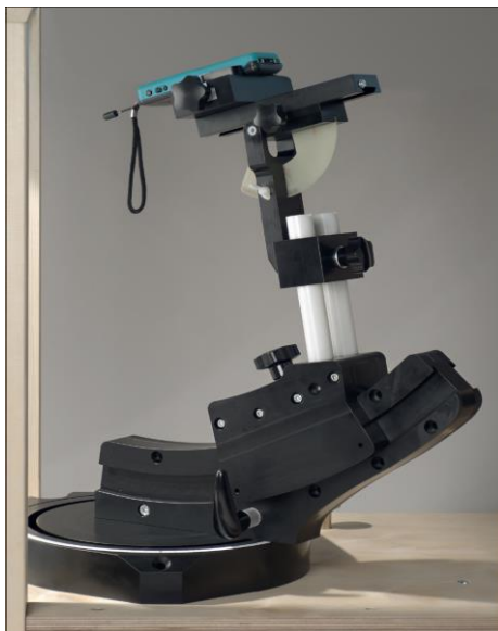
F-2. Device Holder for Transmitters
