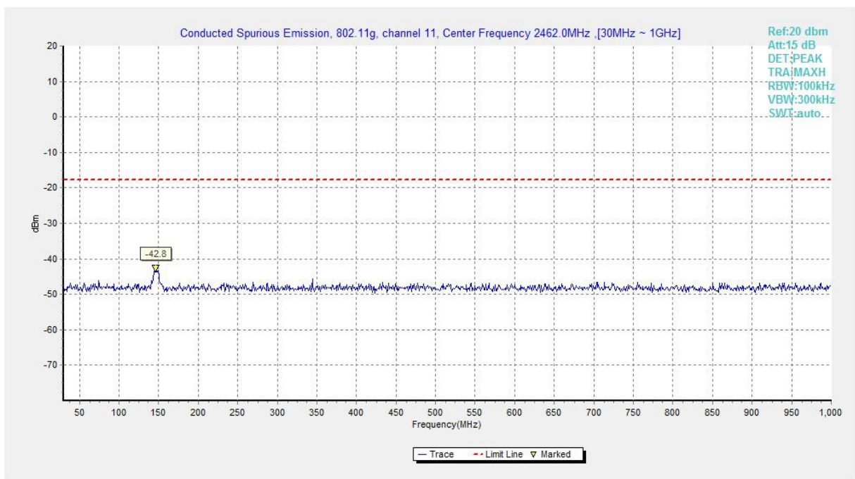
Fig.A.6.1.42 Transmitter Spurious Emission - Conducted (802.11g, Ch11, 30 MHz-1 GHz)
