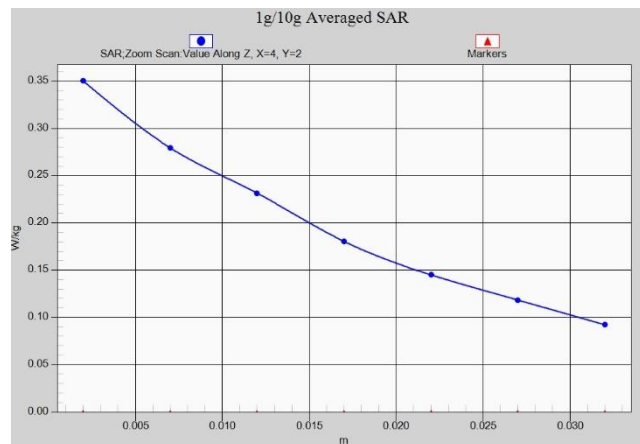
Fig. 1-1 Z-Scan at power reference point (GSM850)
