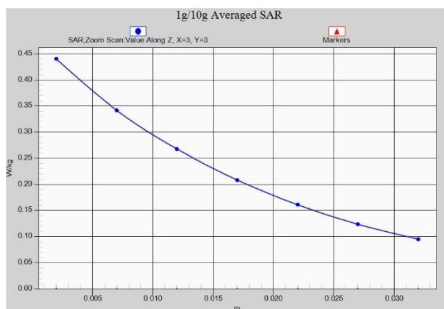
Fig. 1-16 Z-Scan at power reference point (LTE Band13)
