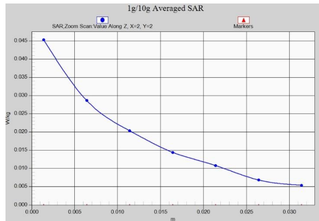
Fig. 1-13 Z-Scan at power reference point (LTE B4 Head)
