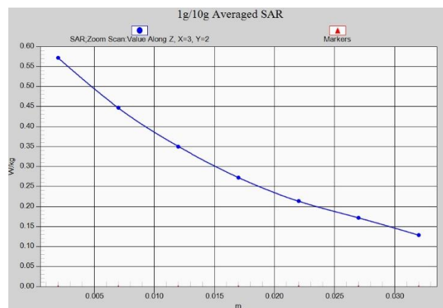
Fig. 1-6 Z-Scan at power reference point (WCDMA850 Body)
