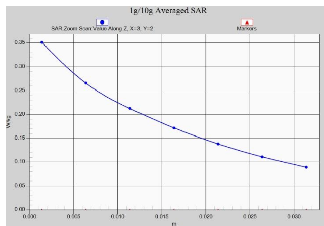
Fig. 1-5 Z-Scan at power reference point (WCDMA850 Head)
