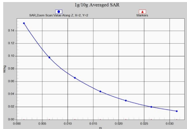
Fig. 1-7 Z-Scan at power reference point (WCDMA1700 Head)
