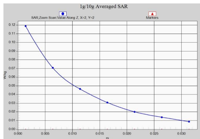
Fig. 1-9 Z-Scan at power reference point (WCDMA1900 Head)
