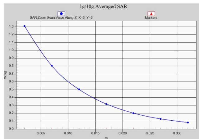
Fig. 1-14 Z-Scan at power reference point (LTE B4 Body)
