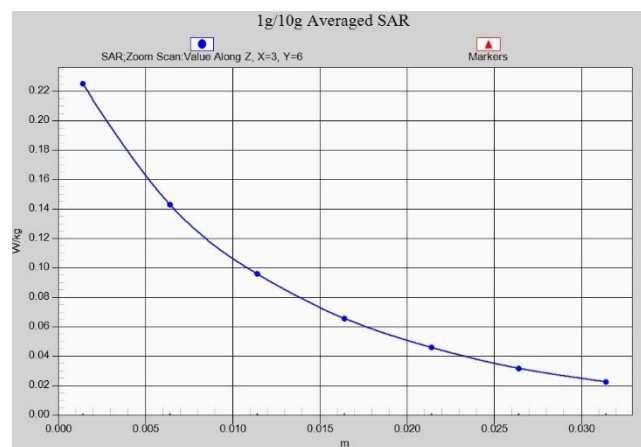
Fig. 1-20 Z-Scan at power reference point (LTE B12 Body)
