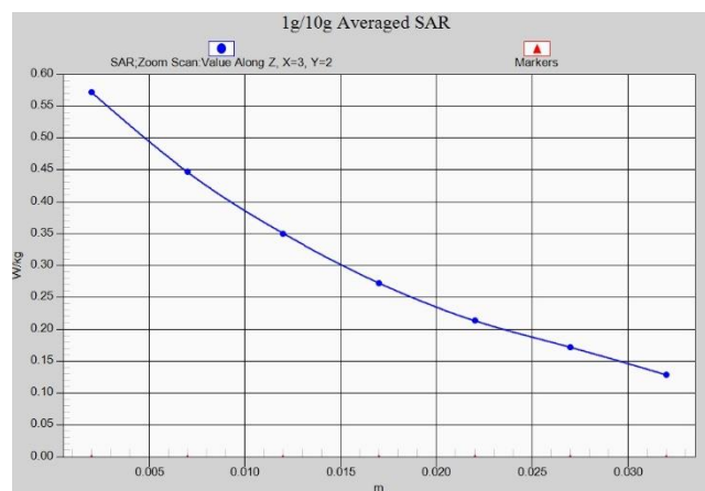
Fig. 1-6 Z-Scan at power reference point (WCDMA850 Body)
