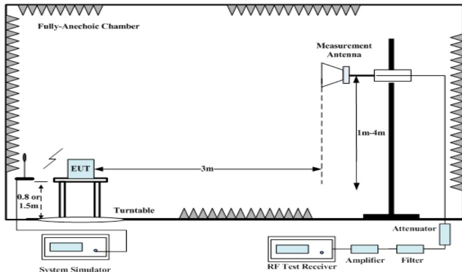
1. The EUT is then put into continuously transmitting mode at its maximum power level during the test. And the maximum value of the receiver should be recorded as (Pr).
