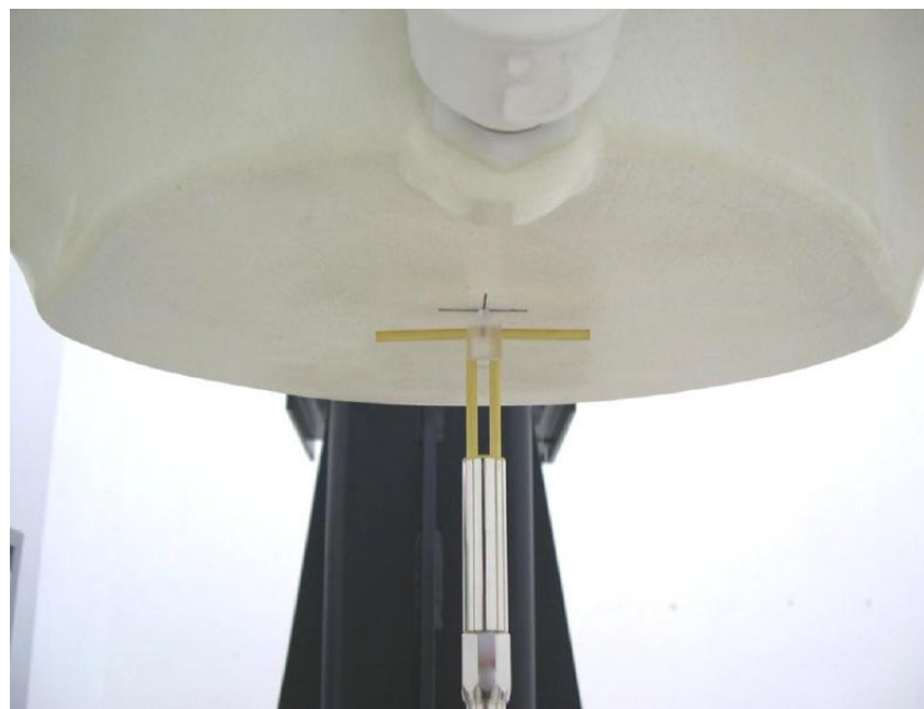
Picture 4 Photo of Dipole Setup
