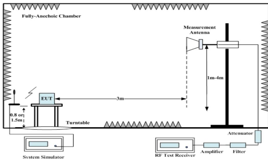
2. The EUT is then put into continuously transmitting mode at its maximum power level during the test. And the maximum value of the receiver should be recorded as (Pr).
