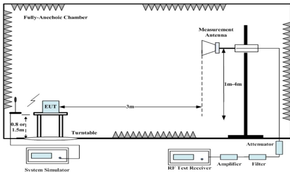
1. The EUT is then put into continuously transmitting mode at its maximum power level during the test. And the maximum value of the receiver should be recorded as (Pr).
