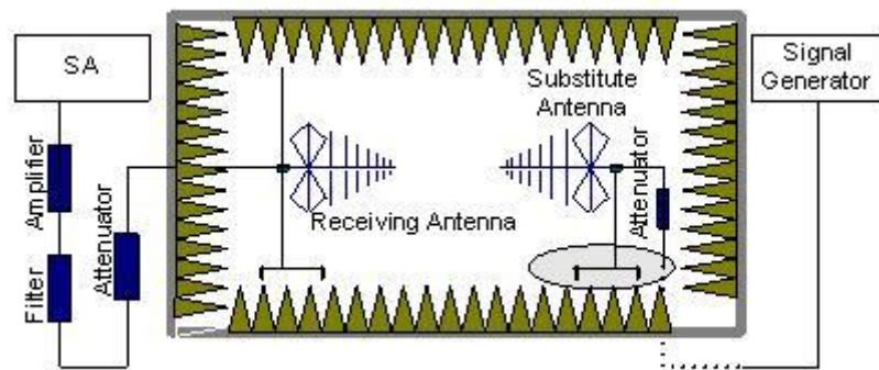
In the chamber, a substitution antenna for the frequency band of interest is placed at the reference point of the chamber. An RF Signal source for the frequency band of interest is connected to the substitution antenna with a cable that has been constructed to not interfere with the radiation pattern of the antenna. A power ( $P_{Mea}$ ) is applied to the input of the
