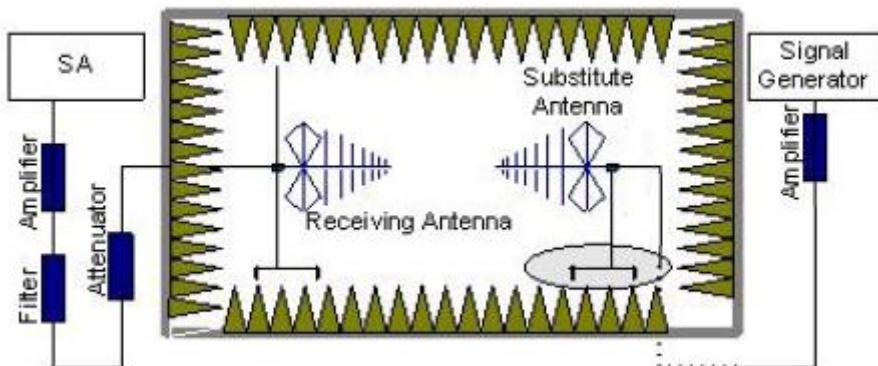
In the chamber, a substitution antenna for the frequency band of interest is placed at the reference point of the chamber. An RF Signal source for the frequency band of interest is
