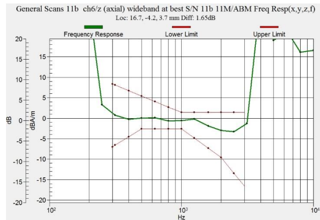
Figure C.10 Frequency Response of WiFi-2.4G
