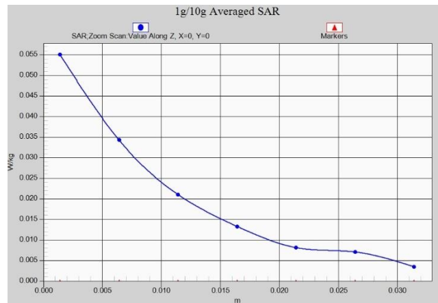
Fig. 1-13 Z-Scan at power reference point (WIFI 2.4G Head)
