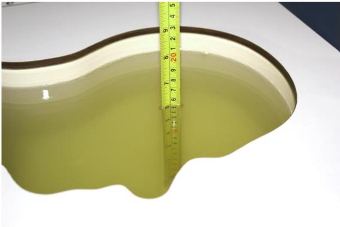
Picture 7-7 Liquid depth in the Head Phantom (2600 MHz)
