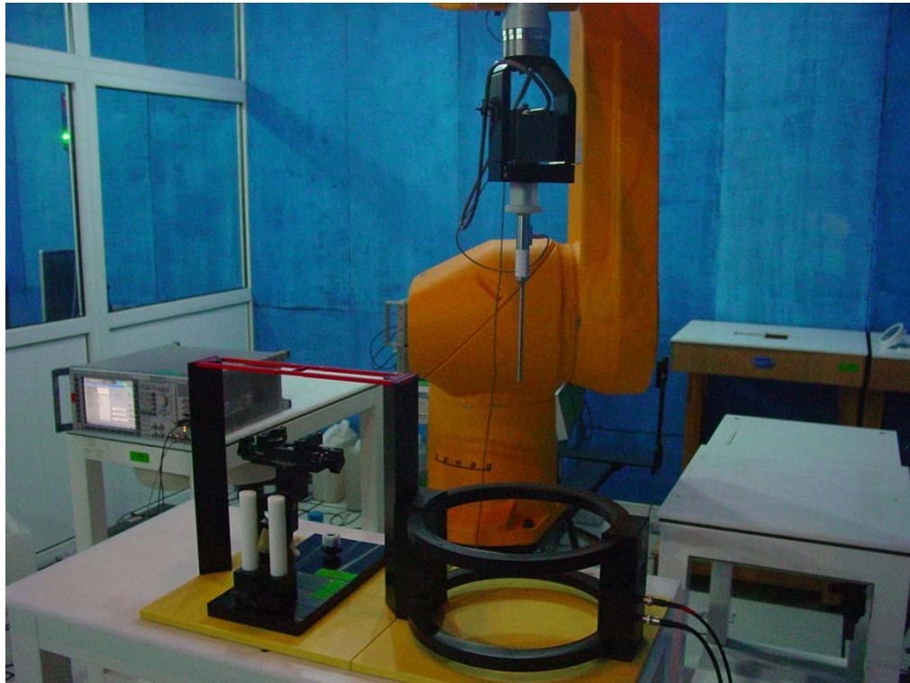
Picture A1: HAC T-Coil System Layout
