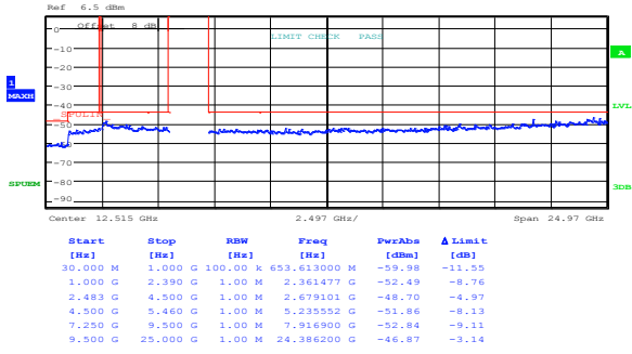
Figure 8.5-35: Conducted peak spurious emissions within restricted bands for 802.11n, high channel at minimum rate
