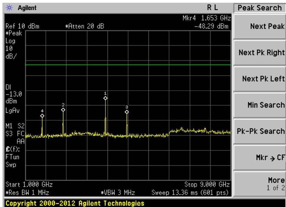
Test Mode: GSM 850 CH 190
