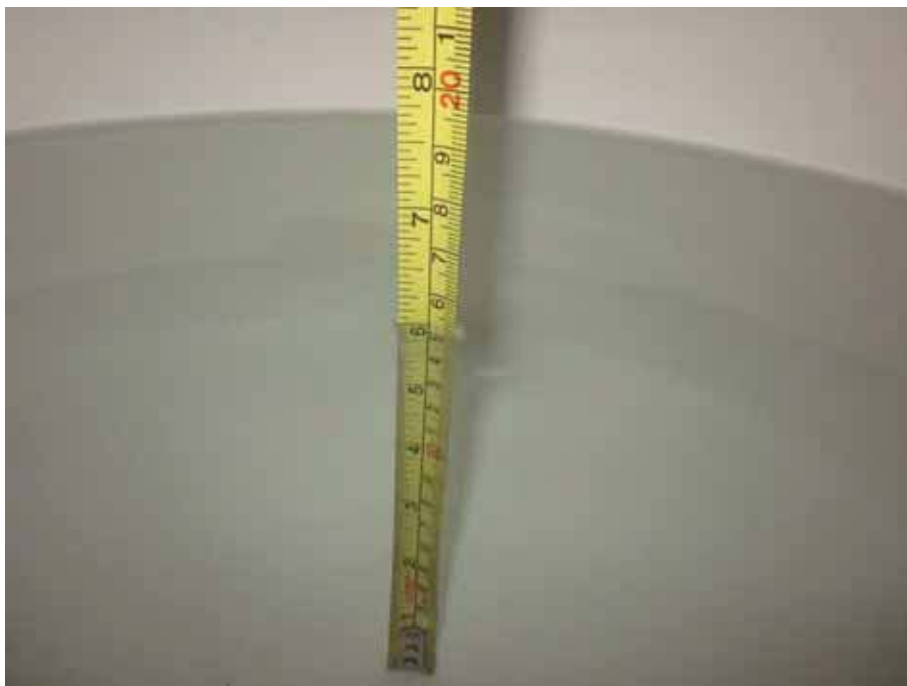
Figure 10.2: Liquid depth in the Flat Phantom ( 900MHz, 1900MHz 15.2cm)
