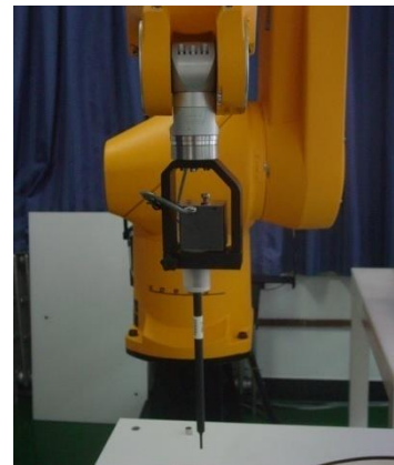
Picture C.3 E-field Probe
