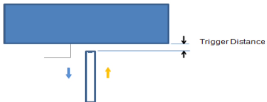
Picture: Proximity sensor triggering distances assessment (Tops)
