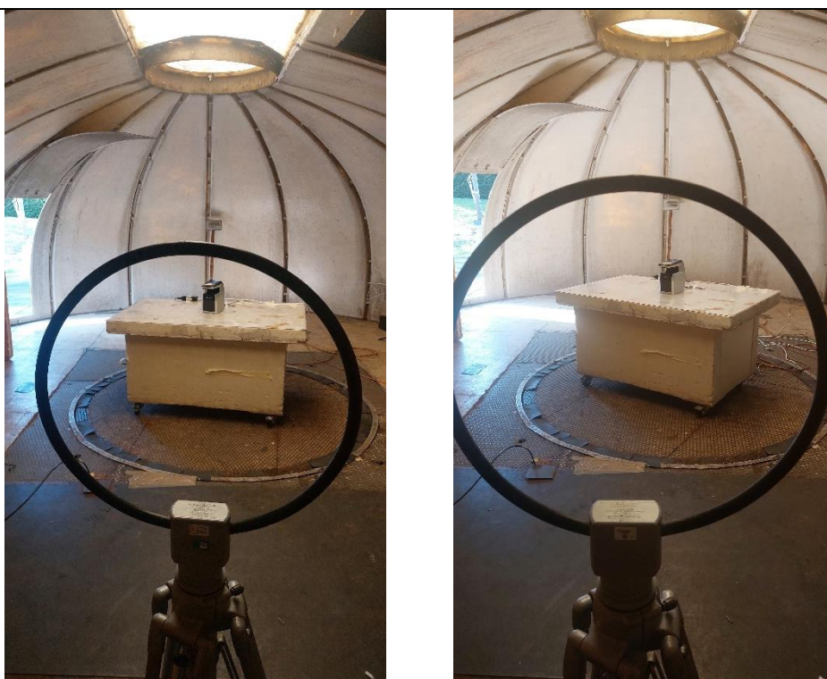
Photo of Field strength within the band 13.110-14.010MHz in OATS
