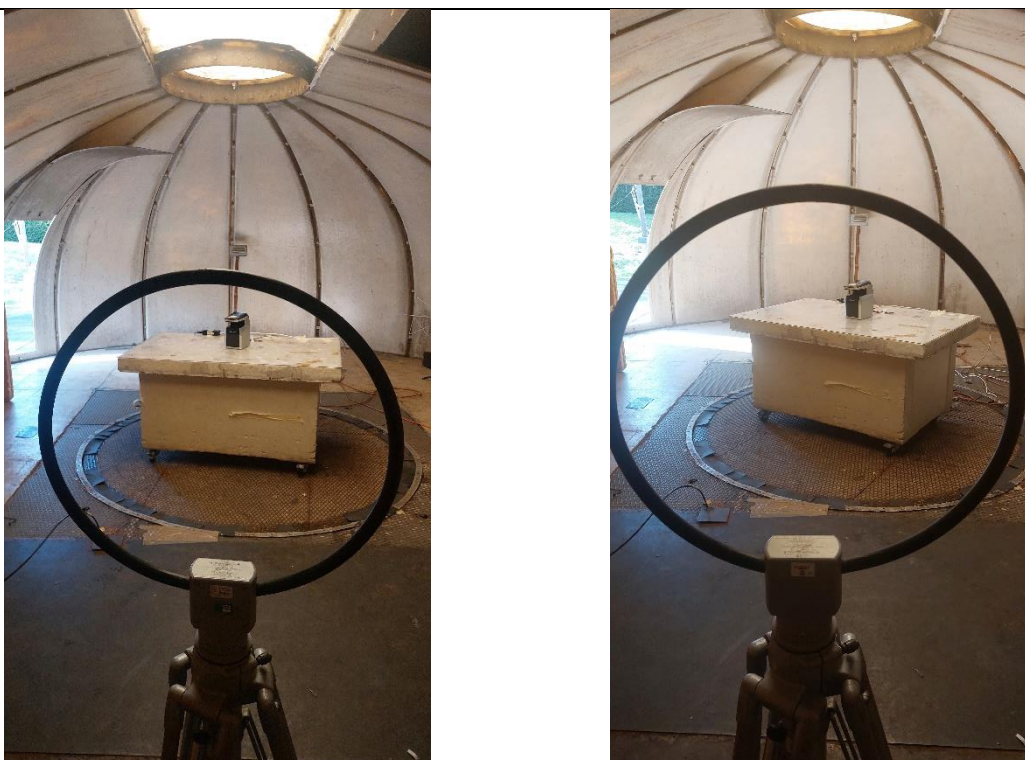
Photo of Field strength within the band 13.110-14.010MHz in Climatic Chamber
