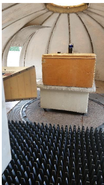
Photo of Field strength outside the band 13.110-14.010MHz
