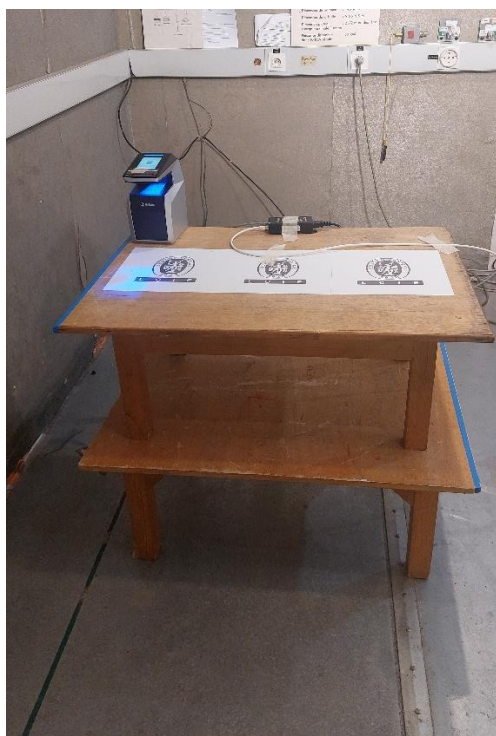
Photo of AC Power Line Conducted Emissions
