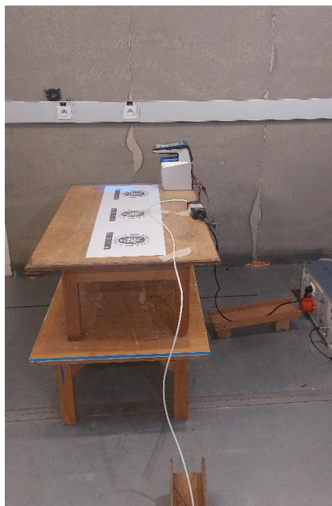
Photo of AC Power Line Conducted Emissions
