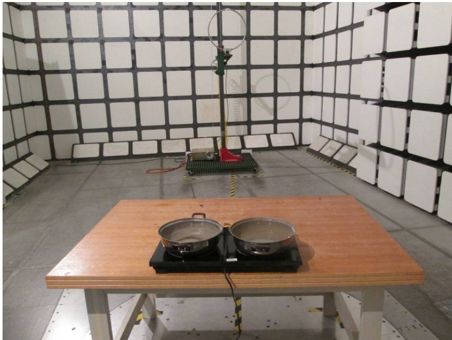
Radiated Emissions - Rear View (90 kHz-30 MHz)
