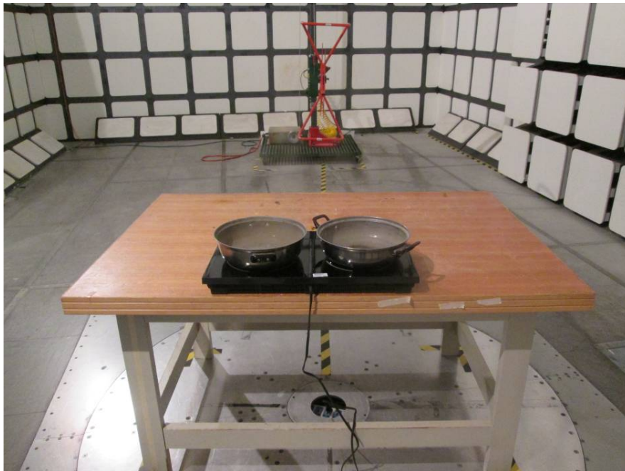
Radiated Emissions - Rear View (30 MHz-1GHz)
