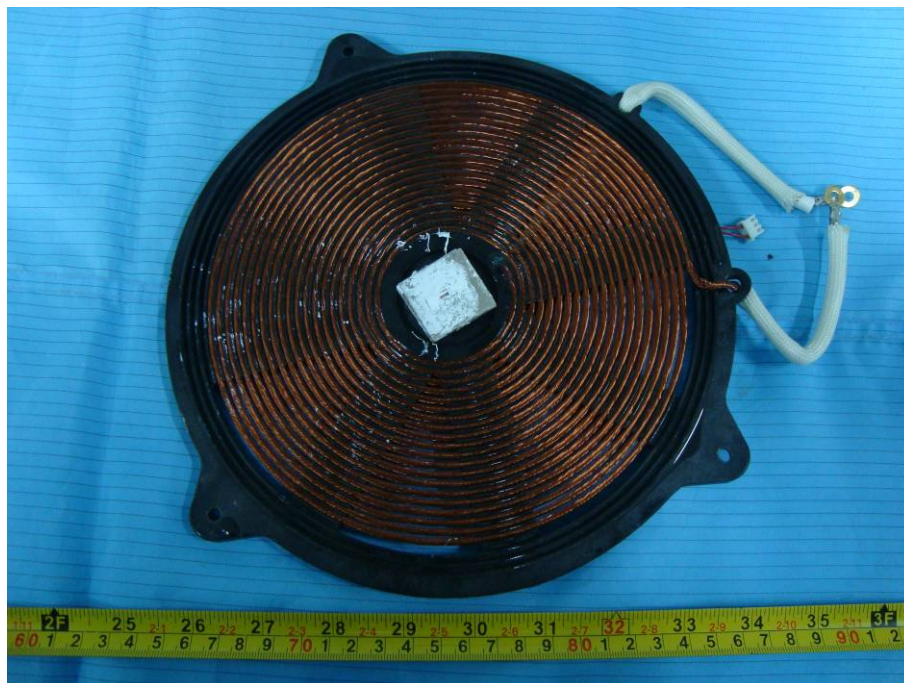
EUT – Induction Coil Front View
