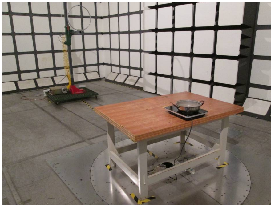
Radiated Emissions - Rear View (90 kHz-30 MHz)
