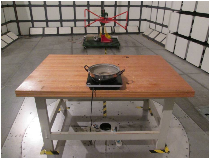
Radiated Emissions - Rear View (30 MHz-1GHz)
