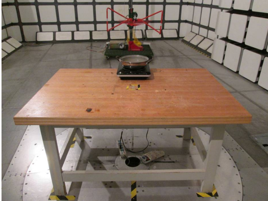
Radiated Emissions - Front View (30 MHz-1GHz)
