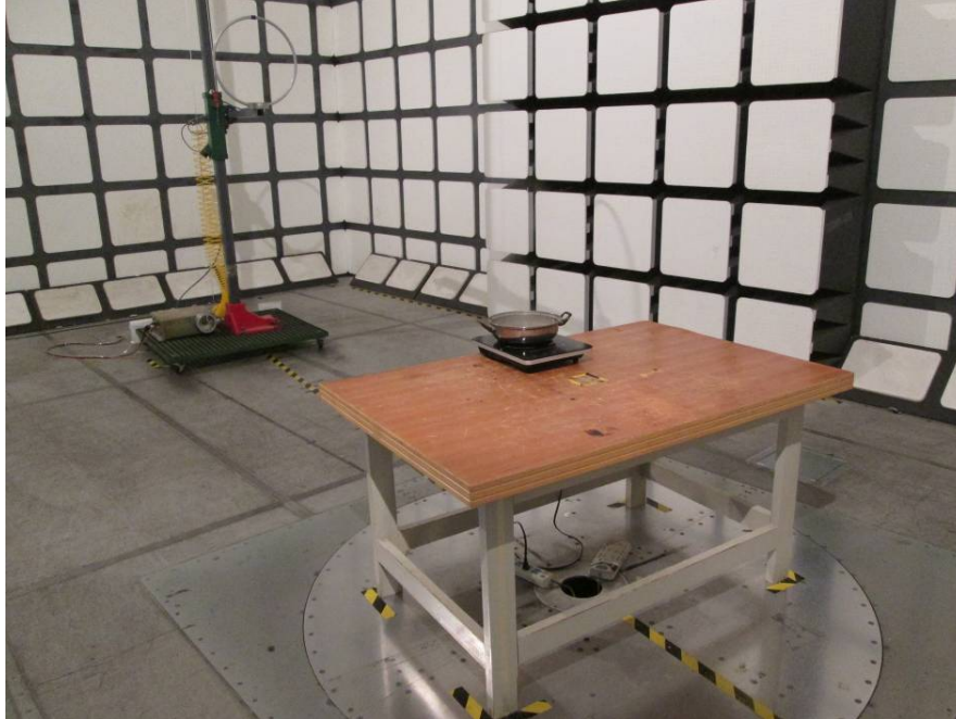
Radiated Emissions - Front View (90 kHz-30 MHz)
