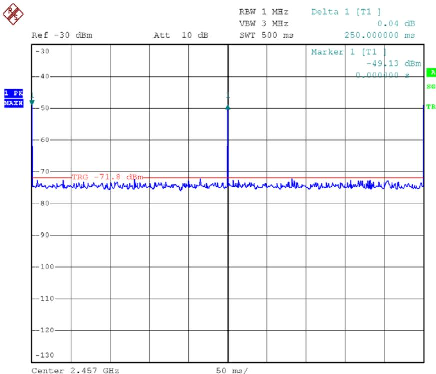
Average Factor Plot – Pursuant to FCC Part 15 Section 15. 249 Requirement (Pass/Fail)
