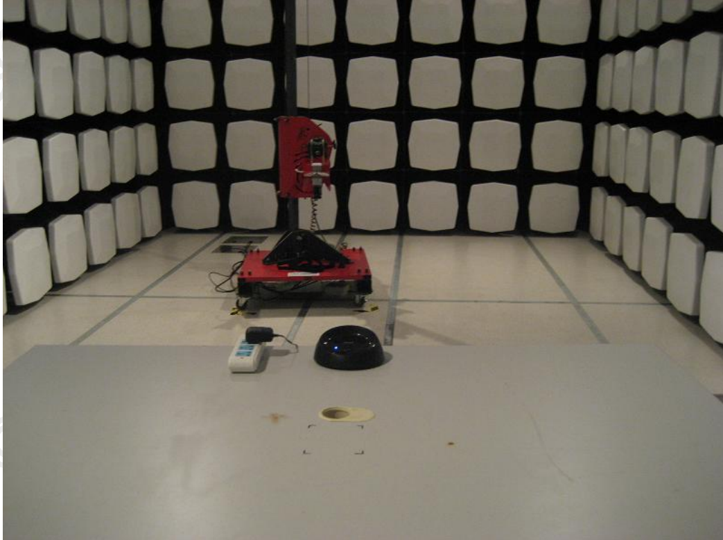
Measurement of Radiated Emission Test Set Up
