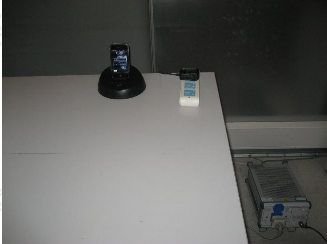
Measurement of Conducted Emission Test Set Up
