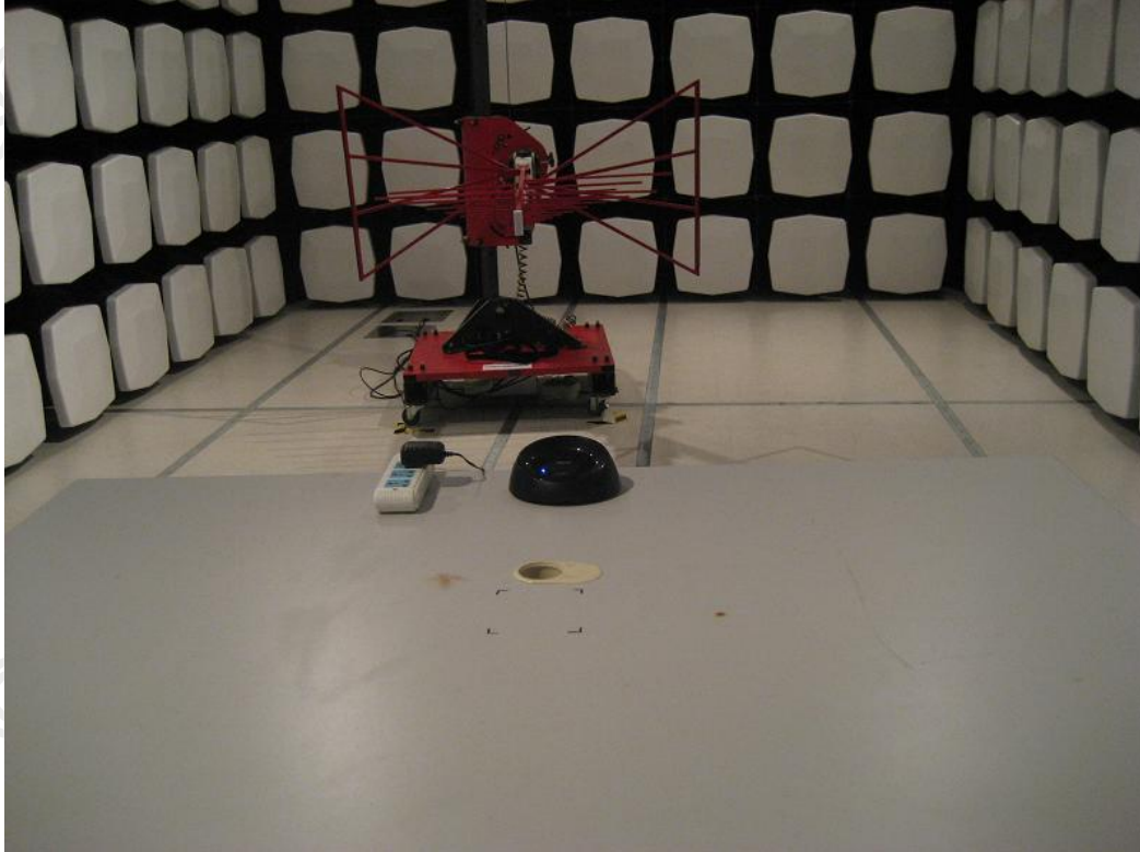
Measurement of Radiated Emission Test Set Up
