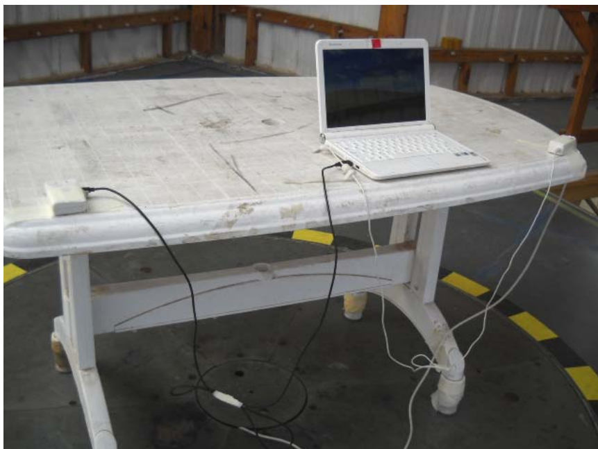
Photograph No.4 Setup for radiated emission measurements at OATS, EUT close view
