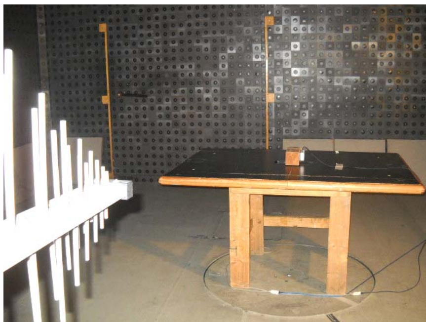
Photograph No.2 Setup for out of band spurious radiated emission measurements in 30 -1000 MHz in the anechoic chamber
