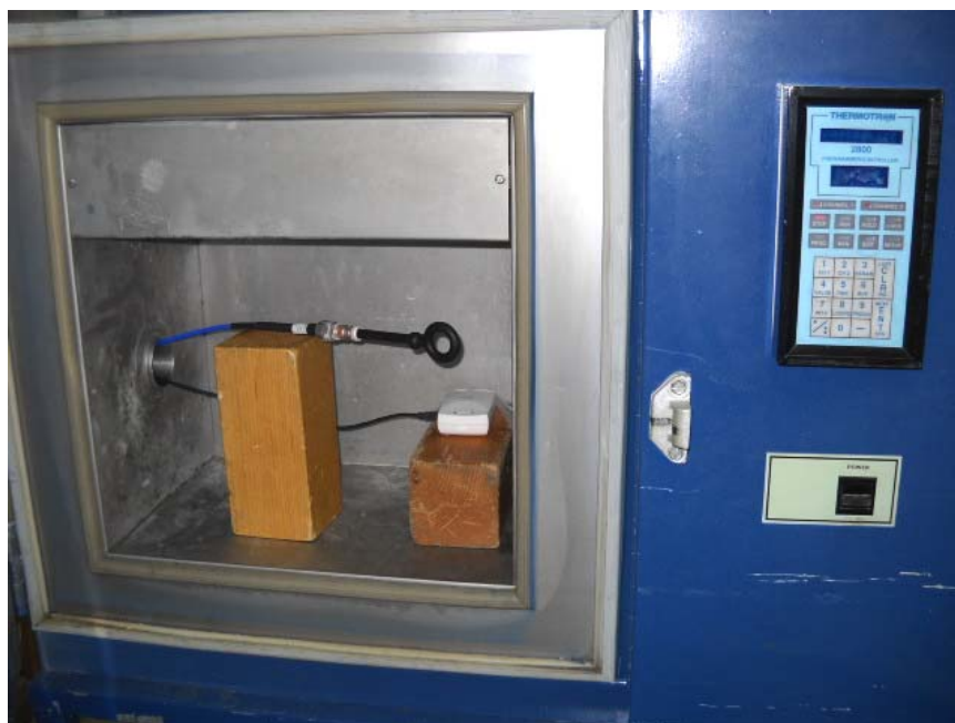
Photograph No.6 Setup for frequency stability test and occupied bandwidth test
