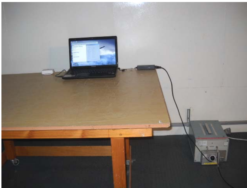
Photograph No.7 Setup for conducted emission measurements in shielded room
