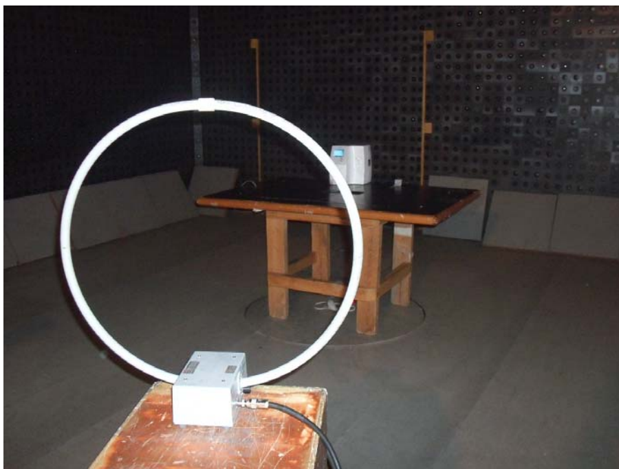
Photograph No.2 Setup for out of band radiated emission measurements below 30 MHz in the anechoic chamber
