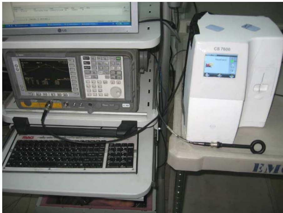
Photograph No.7 Setup for occupied bandwidth test
