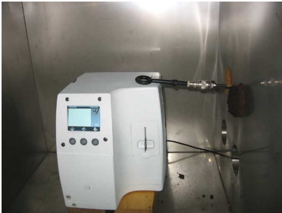
Photograph No.6 Setup for frequency stability test
