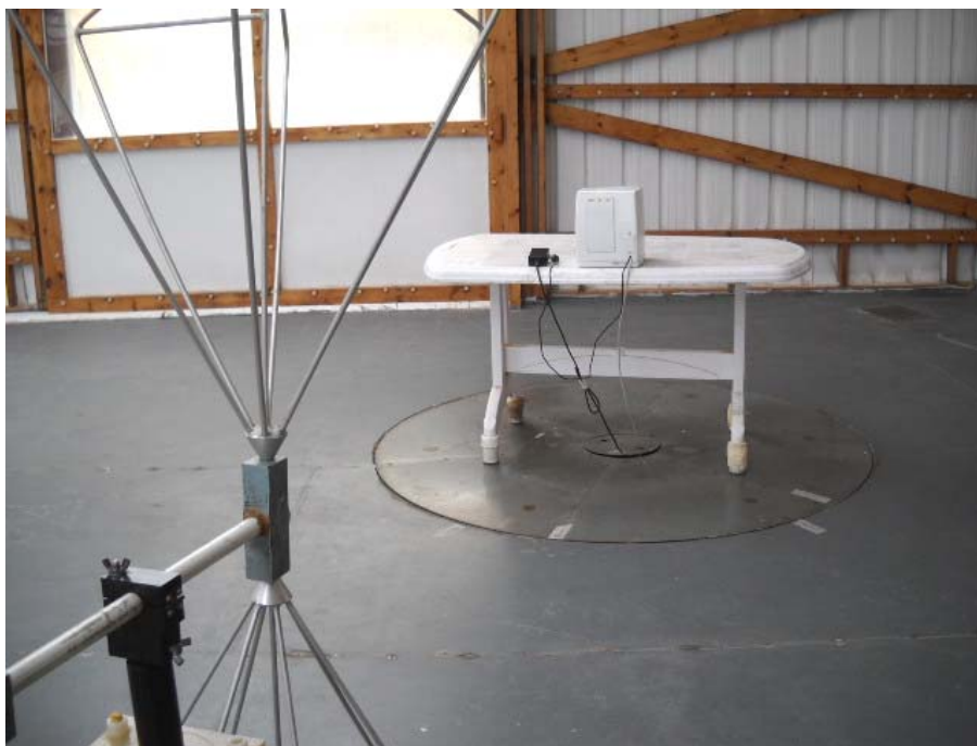
Photograph No.3 Setup for out of band radiated emission measurements above 30 MHz at OATS, general view
