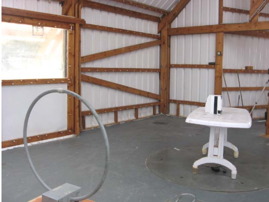
Photograph No.1 Setup for in band radiated emission measurements at OATS
