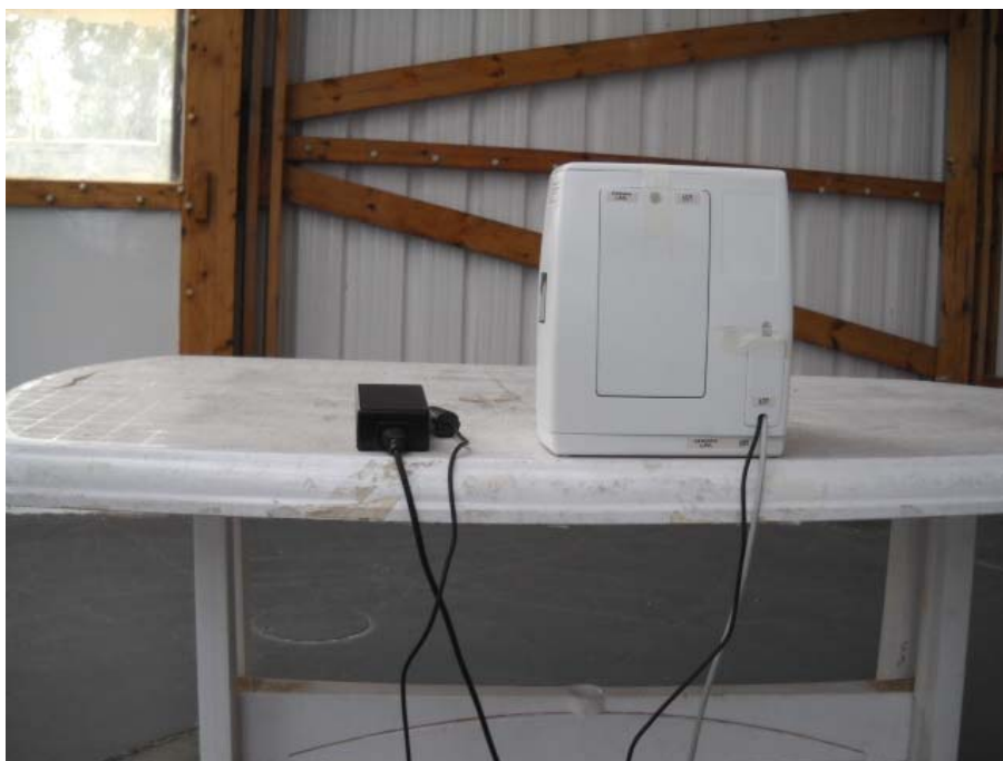
Photograph No.4 Setup for out of band radiated emission measurements above 30 MHz at OATS, EUT view
