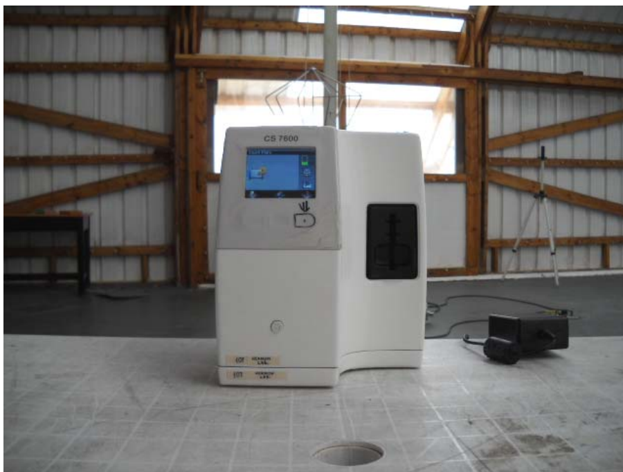
Photograph No.5 Setup for out of band radiated emission measurements above 30 MHz at OATS, EUT view
