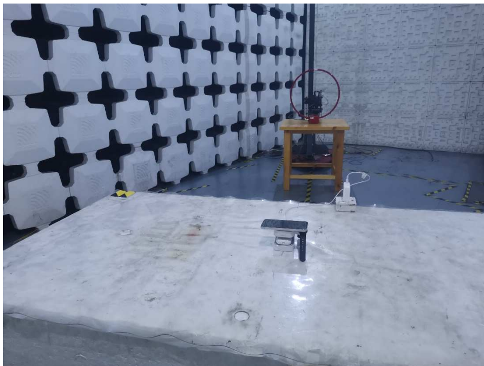
Photograph 1: Set-up photo for Radiated Spurious Emission, Below 30MHz
