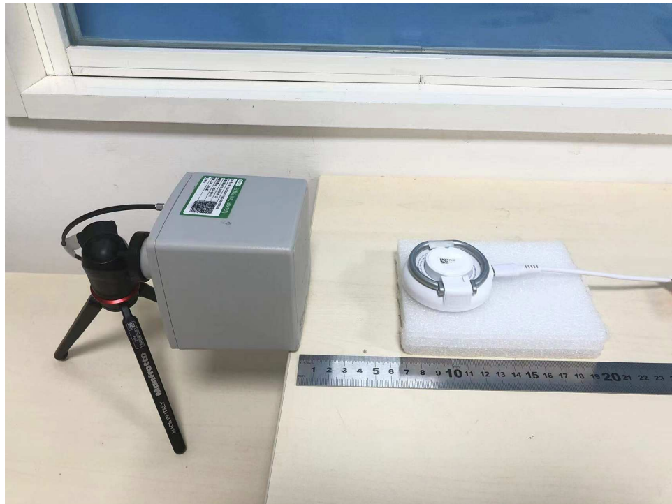
Photograph 1: Set-up photo for RF exposure
