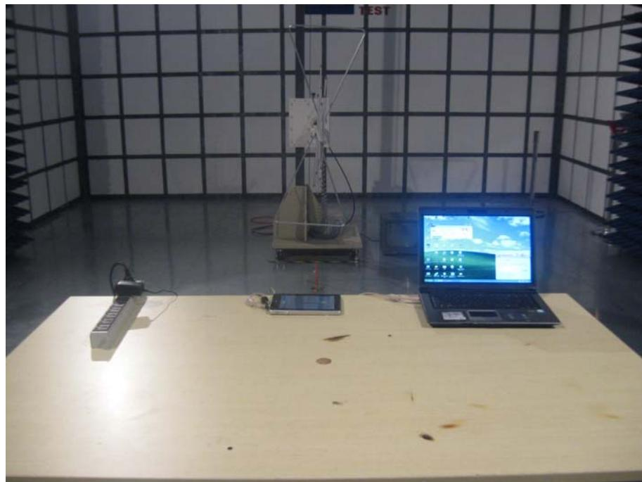
**Radiation Emission Test Setup ( 1-6GHz)**
